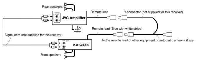
\*3 Firmly attach the ground wire to the metallic body or to the chassis of the car—to the place not coated with paint (if coated with paint, remove the paint before attaching the wire). Failure to do so may cause damage to the receiver.
